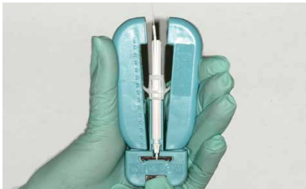
Figure 7. Stripping of the protective outer cladding
