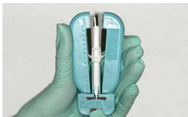
Figure 7. Stripping of the protective outer cladding
